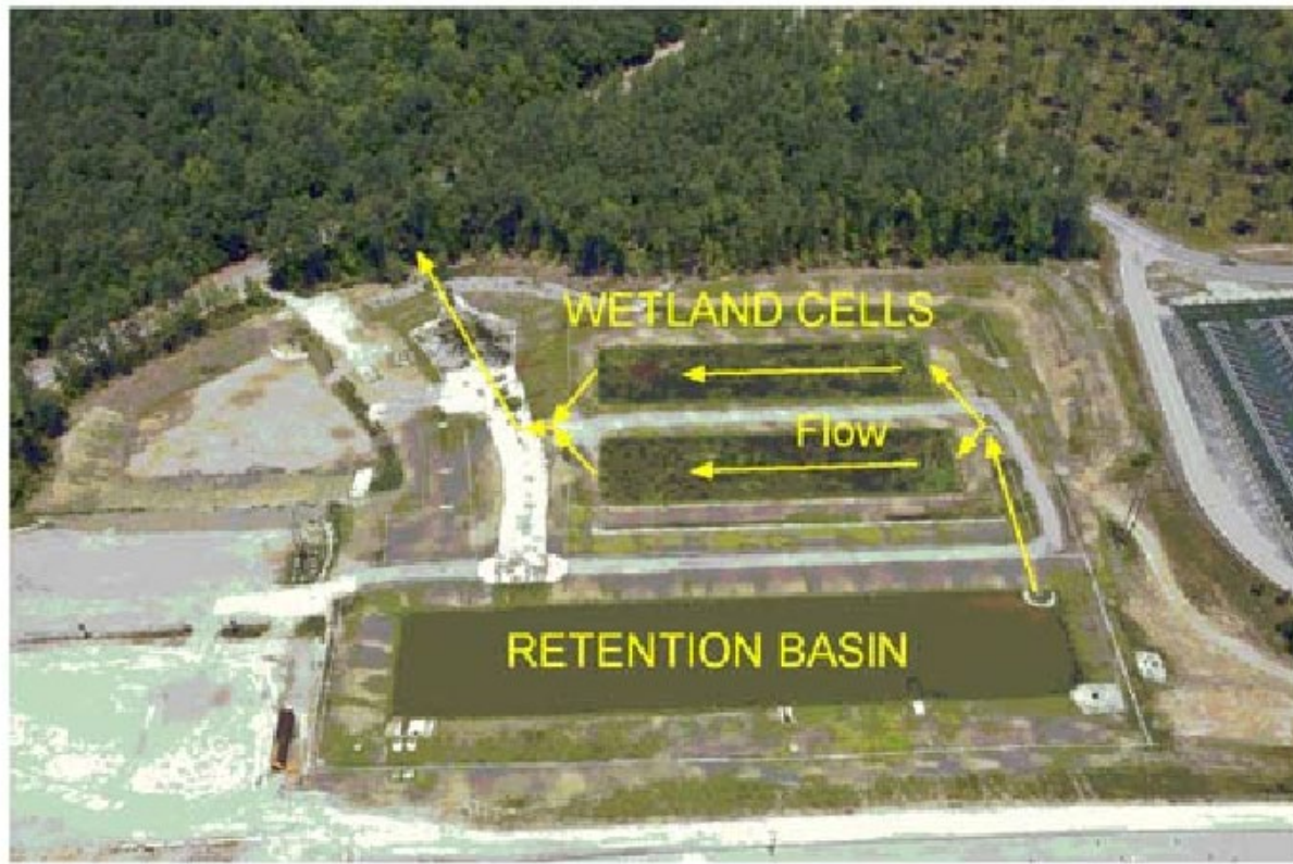
Figure 2. Layout and water flow path through CWTS
